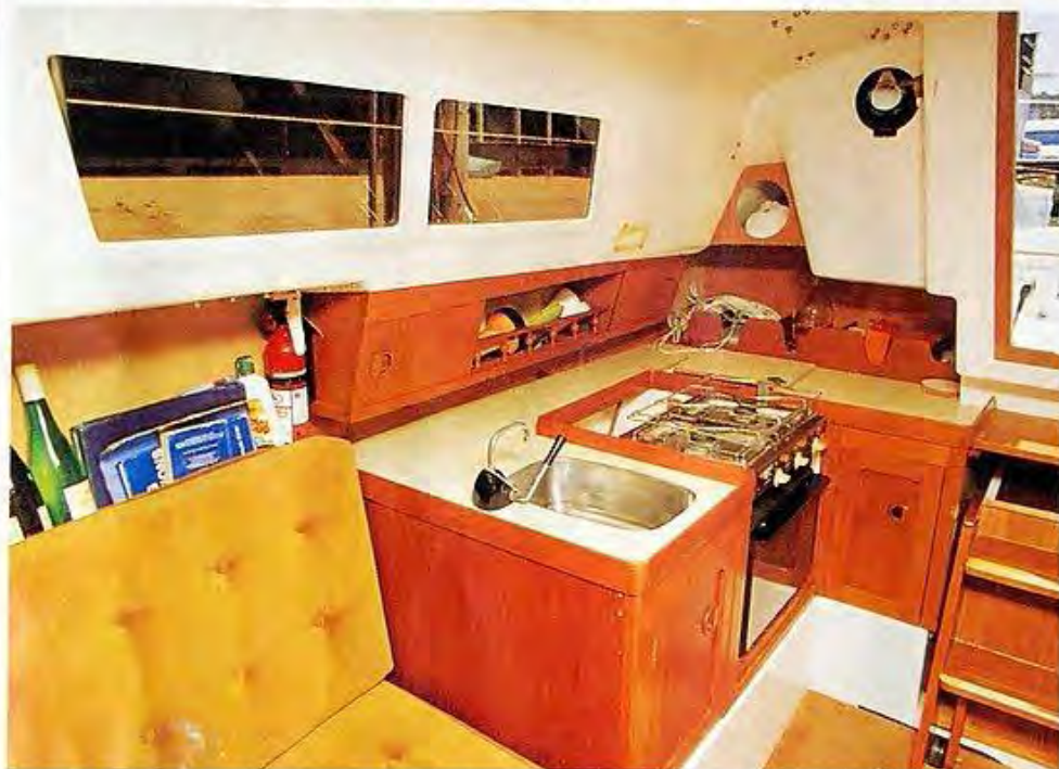
Looking aft the galley features gimble oven and stove and teak faced lockers.
