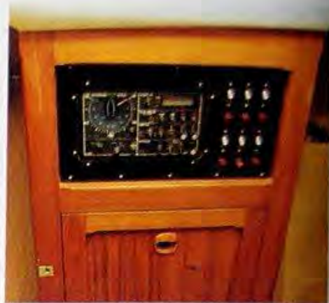
Instrument panel over navigator's table features wind instrument readout.
