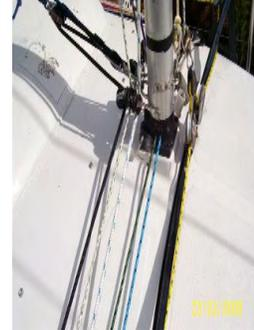
David replaced all his sheets with spectra, changed the jib sheets to a 2:1 arrangement and replaced his vang with a powerful and easy to handle 5:1 setup. He also changed the mainsheet traveller to a 5:1 system as described in the 'Handy Hints' booklet.
