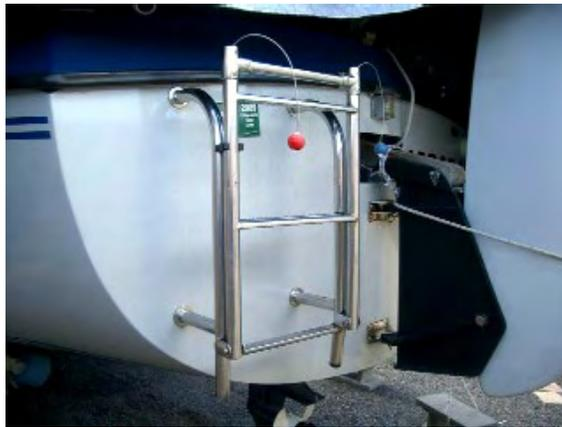
Rigging wire inside each tube attached to the hinge pins at one end and 25mm barrel bead/rope stop balls at the other end, the wires being just the right length so that when the extra rung is lowered it is restrained by the wires & balls.
